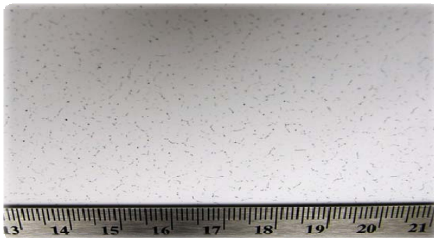
Figure 1 – Vitrium Threading. Opaqueness of whitecoat to show underlying Vitrium bluecoat
